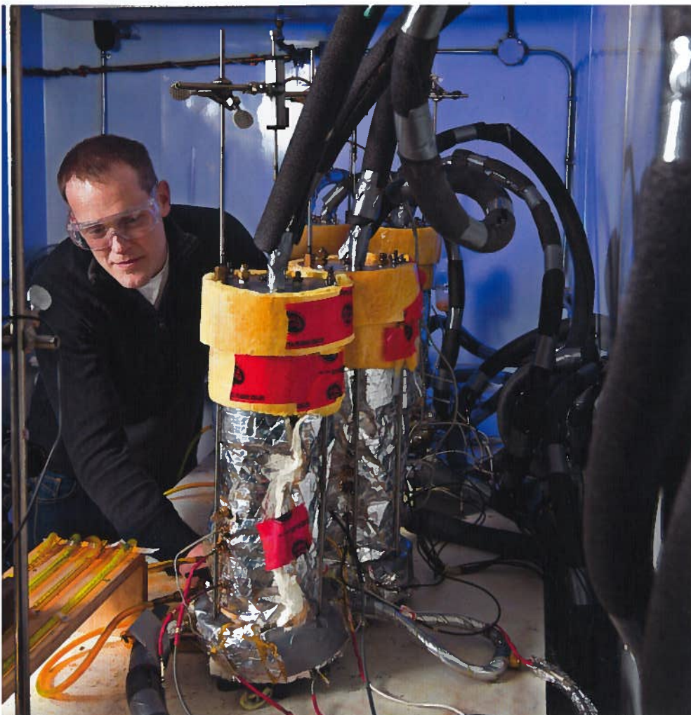
Michael Hendry, a professor in the Department of Civil and Environmental Engineering and associate director of CaRRL, inspects a graduate student's experiment measuring the effects of freeze-thaw cycles.
